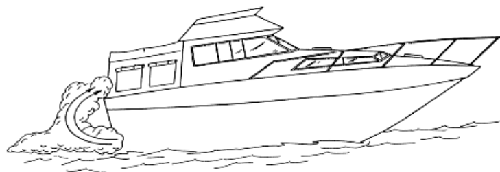
As shown in this figure, certain canvas configurations, such as side curtains, and position of hatches can increase backdrafting.
