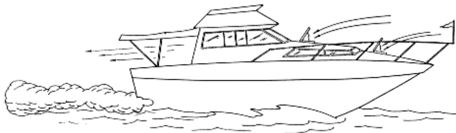
This figure illustrates desired airflow through the boat.
